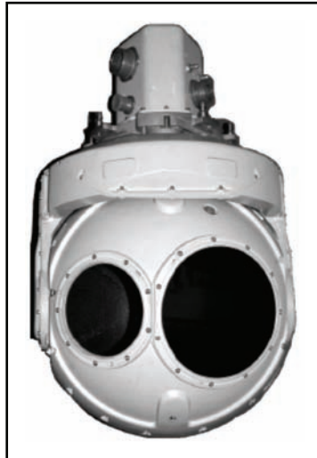
Figure 2-3. Hunter multi-mission optronic stabilized payload
